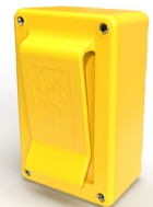
Back of the P2P VibraTag has a clip to attach it to clothing.
