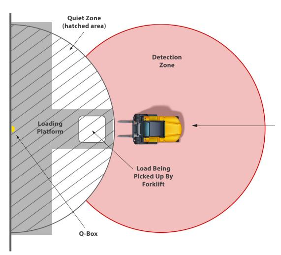
As the forklift approaches the loading platform to pick up the load, the detection zone of the ZoneSafe system is masked preventing detection of pedestrian workers and the ZoneSafe system alarm going off.
